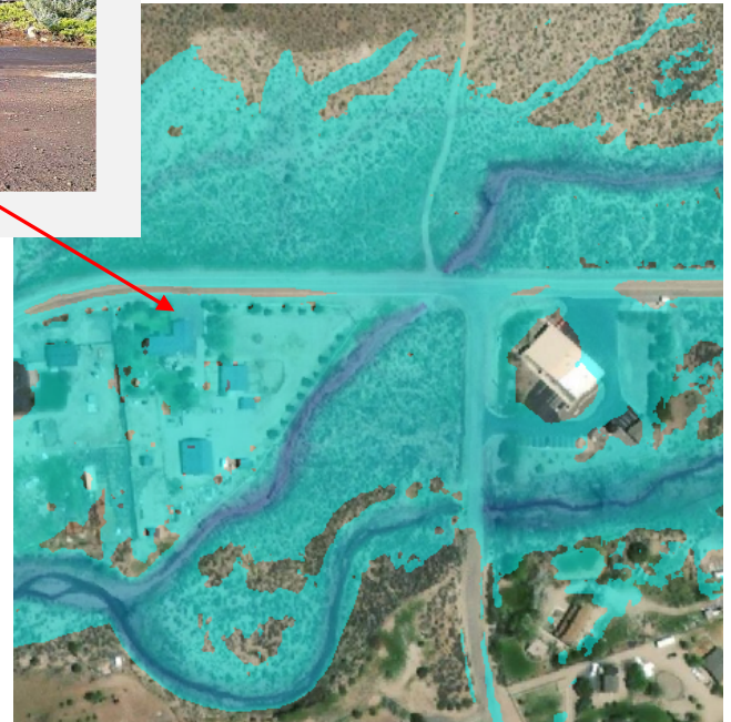
Figure 4: Home Flooded During 8/6/2014 Flash Flood, Compared to HEC-RAS Model Results
